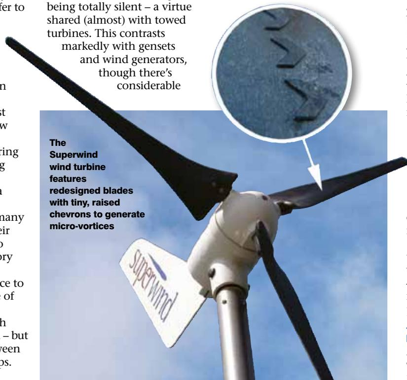
The Superwind wind turbine features redesigned blades with tiny, raised chevrons to generate micro-vortices
