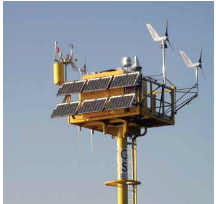
Superwind 350s help power a buoy in the Atlantic Ocean. (Searoc)
